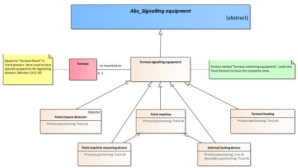
Table 30: Class diagram Turnout signalling equipment
