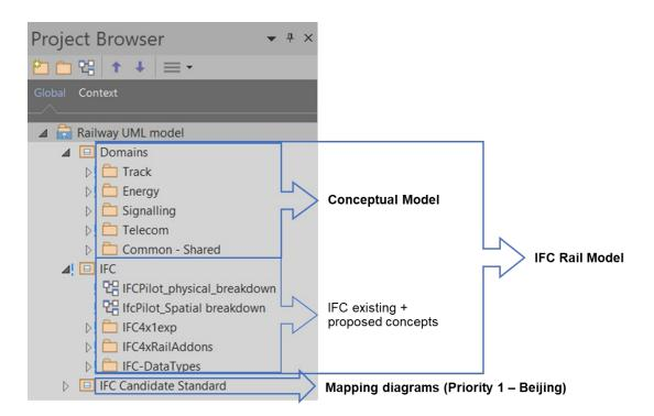
Figure 3 - Structure overview of the Railway UML model
