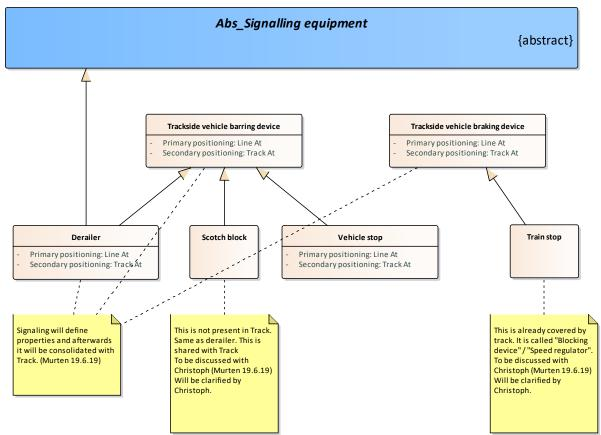
Table 31: Class diagram Vehicle barring/breaking device
