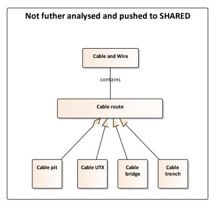
Table 20: Class diagram Cable and Wire
