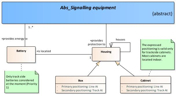
Table 23: Class diagram Housing + Trackside Battery
