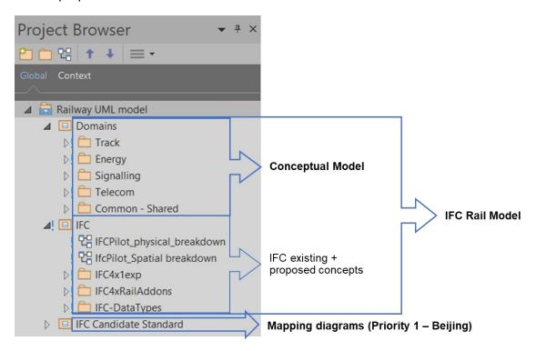
Figure 5 - Package structure of the Railway UML model, with naming convention
