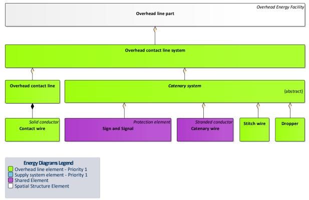
Table 55: Class diagram "Overhead Contact Line System"
